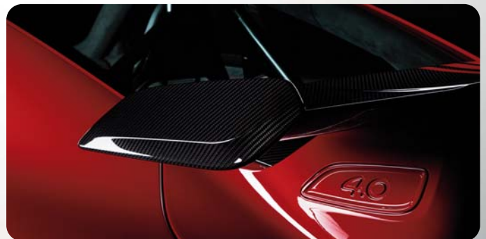
Heckspoilerblenden in der Version Carbon glänzend. Rear spoiler panels in glossy carbon fiber.
