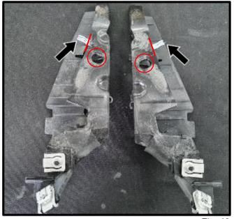
14 Fasten both crash sensors with the original screws and the supplied M6 selflocking nuts as well as the washers 6x20mm.
